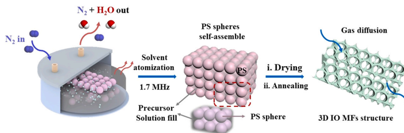
Fig. 1. Illustration of the process flow to fabricate the 3D IO \text{SnO}_2 and \text{Co-SnO}_2 ( \text{Co/Sn} = 1:16, 1:24, \text{ and } 1:48 atom%) MFs.
